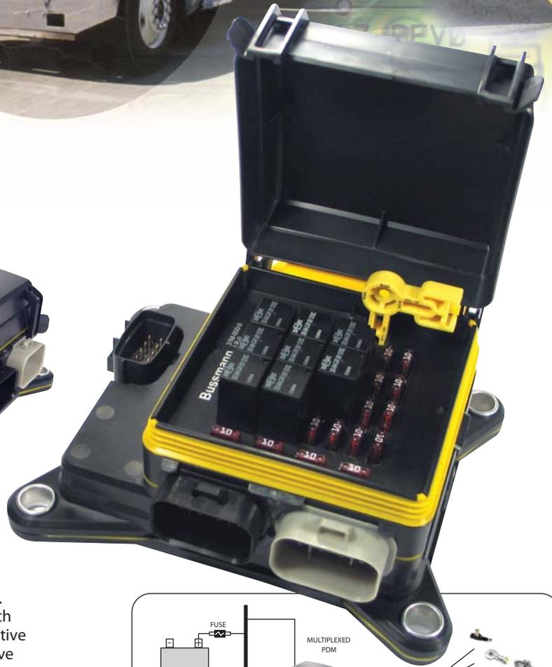
**High Power:** The mVEC uses patented Bussmann VEC 'power grid' technology, ideal for high current circuits, and Vansco Networking Electronics. Each mVEC is rated at 200 Amps, with outputs up to 30A, - 64 outputs are possible with the mVEC. 12 and 24 volt systems are supported.
